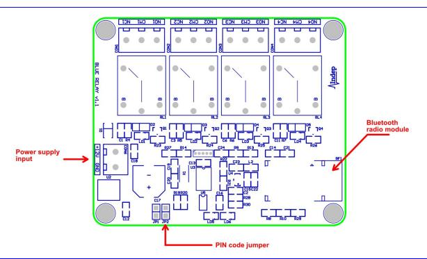
Fig.1 - BLUE RELAY Board layout.
