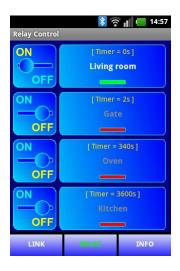
Fig.6 - Screenshots of the RELAY page. Timer value insertion (Bistable: 0s or Monostable: 1 ... 6550s).
